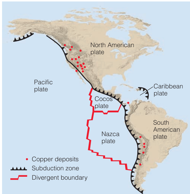
(a) Valuable copper deposits are located along the west coasts of North and South America in association with convergent plate boundaries. The rising magma and associated hydrothermal activity resulting from subduction carried small amounts of copper, which became trapped and concentrated in the surrounding rocks through time.
